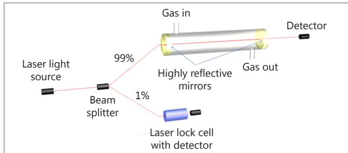
Fig. 3 Principle of CW-CRDS
