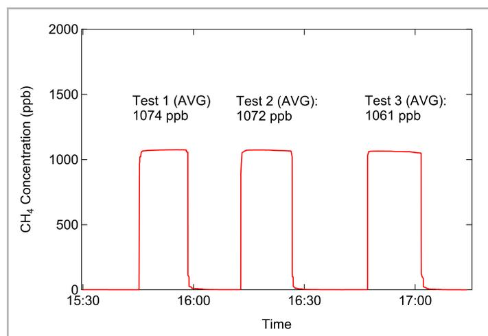
Fig. 3 Repeatability test with a  $\sim 1$  ppm  $\text{CH}_4$  in  $\text{H}_2$  sample using a Prismatic 2 CRDS analyzer
