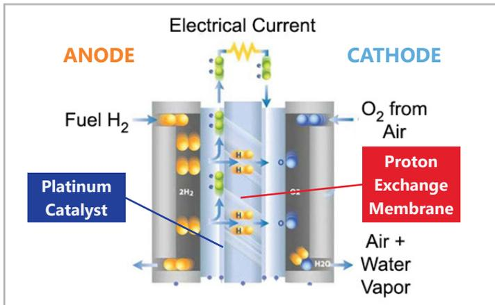
Fig. 1 Schematic and principle of operation of a PEM fuel cell
